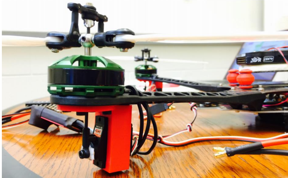
Figure 1: Variable pitch quadrotor concept designed by the Georgia Institute of Technology (image permission requested)
